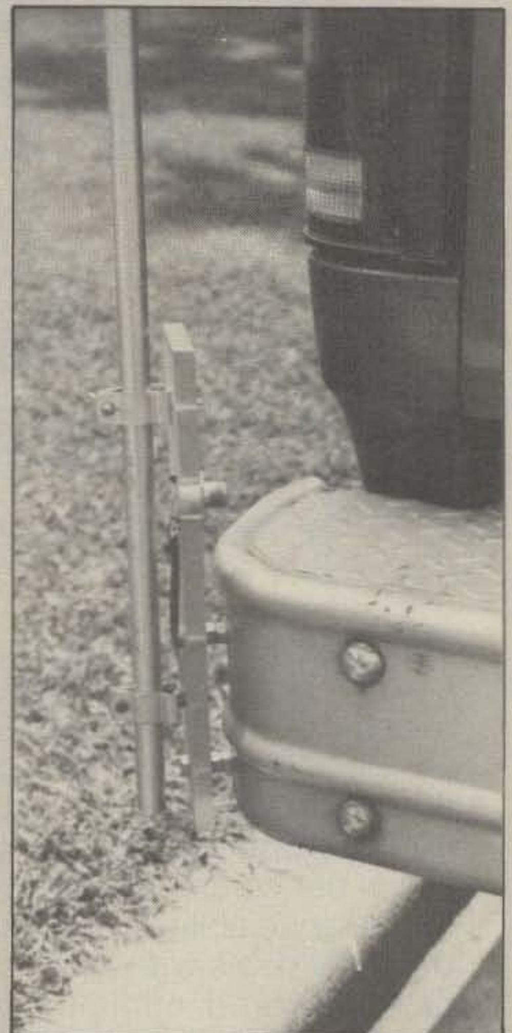
The completed bumper mount on the author's pickup truck.
